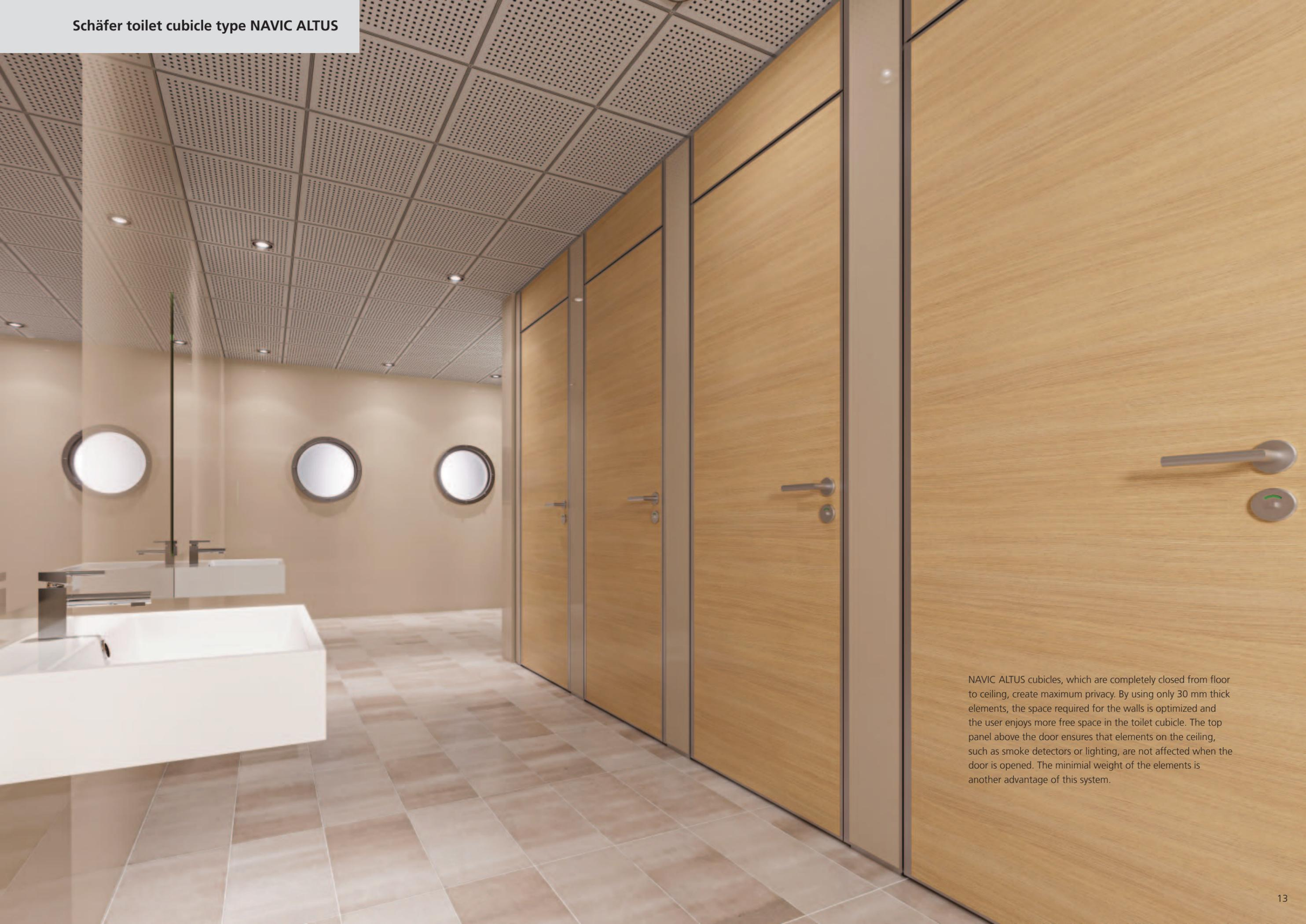
NAVIC ALTUS cubicles, which are completely closed from floor to ceiling, create maximum privacy. By using only 30 mm thick elements, the space required for the walls is optimized and the user enjoys more free space in the toilet cubicle. The top panel above the door ensures that elements on the ceiling, such as smoke detectors or lighting, are not affected when the door is opened. The minimal weight of the elements is another advantage of this system.
